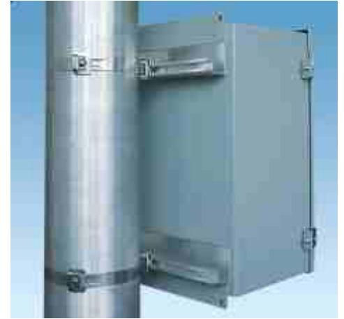
A panel is attached with Easy Mount hardware and support channels. Band and buckle secure the box to round, rectangular or flanged posts.
